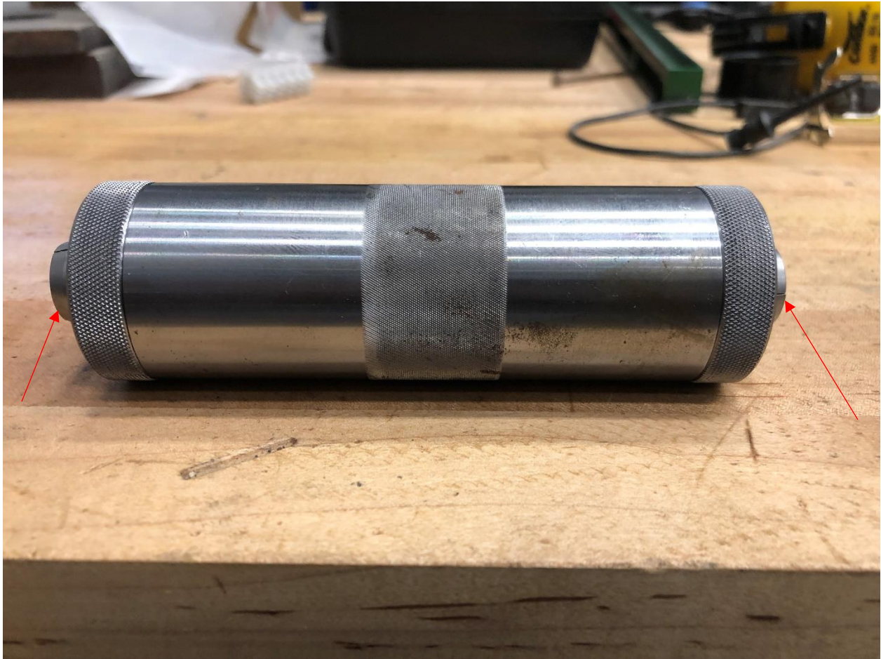
Figure 1. 0.5-in Splice Coupler with 1.2-in three-piece wedge (wedge tips indicated by arrows)
