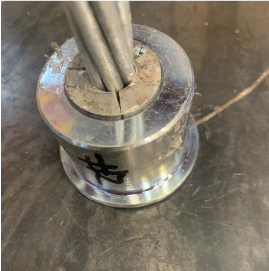
Figure 1. 0.50-in galvanized barrier cable anchorage with galvanized three-piece wedge installed in test machine for static testing
