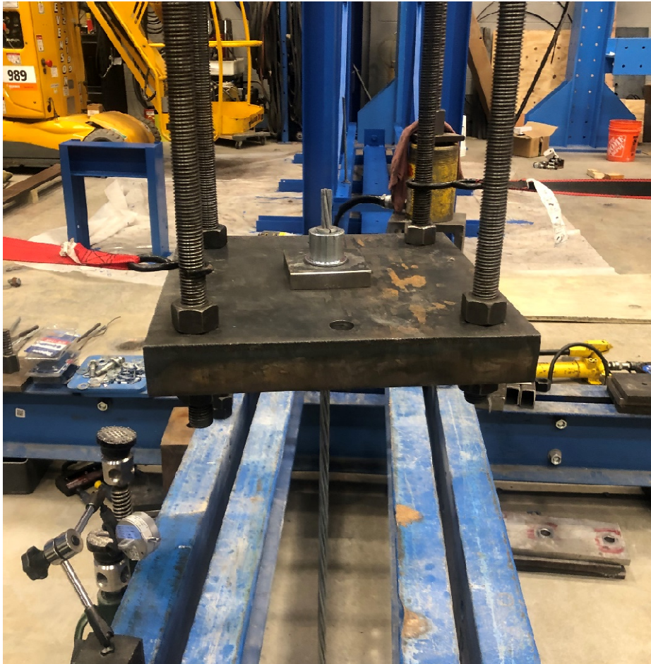
Figure 2. Fatigue anchorage sample bearing on steel plate connected through threaded rods and steel plate to hydraulic actuator
