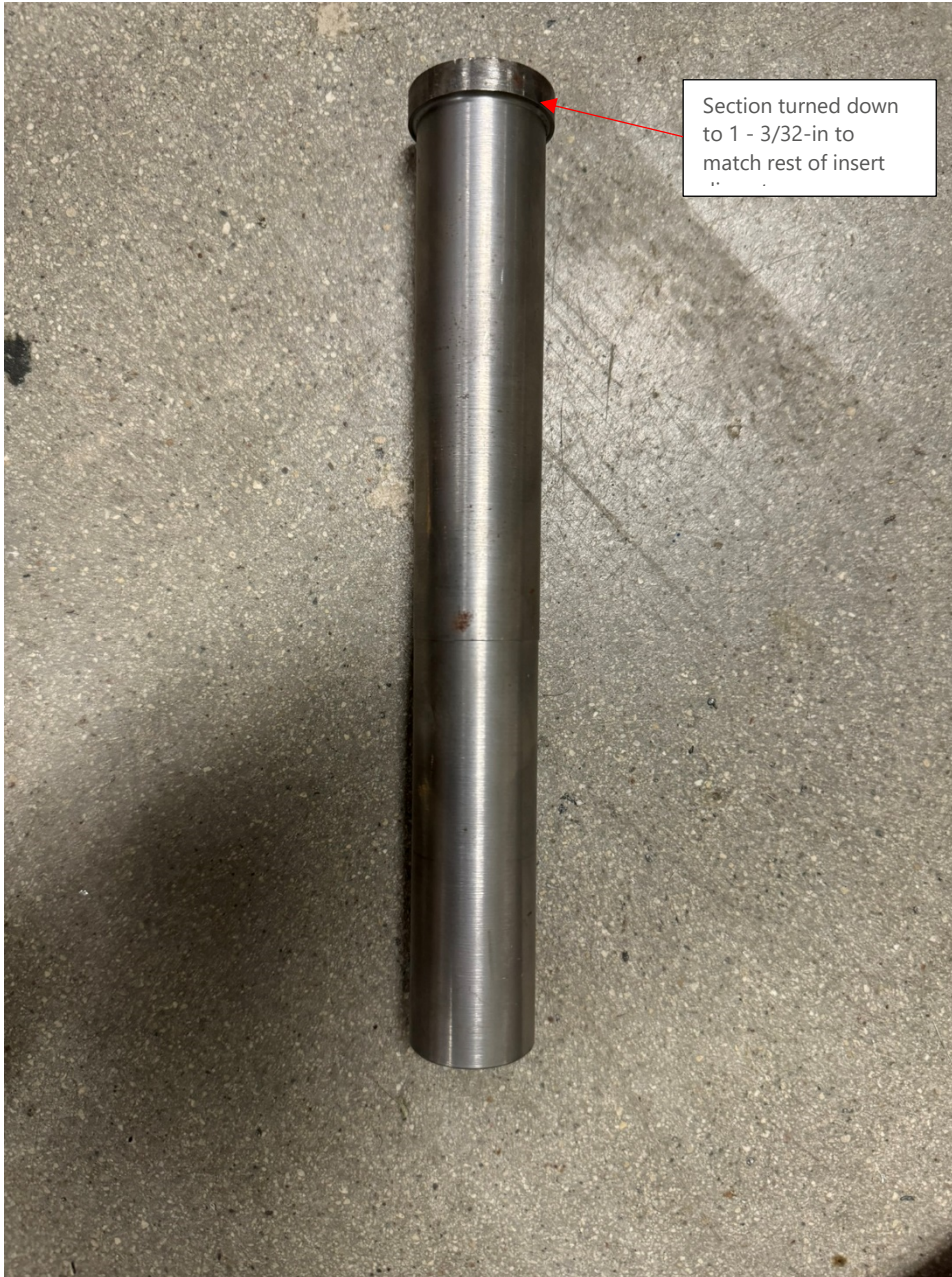
Figure 2. Insert showing section before being turned down to match the diameter of the remaining length of insert.
